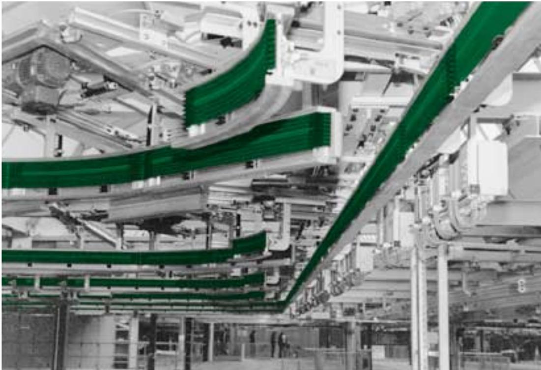
VAHLE U 10 conductors provide power, control and data transmission for automated monorail systems (AMS) in the automotive industry.
