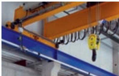
**Powerail enclosed conductor systems**
