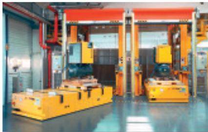
**Contactless Power System (CPS®)**
