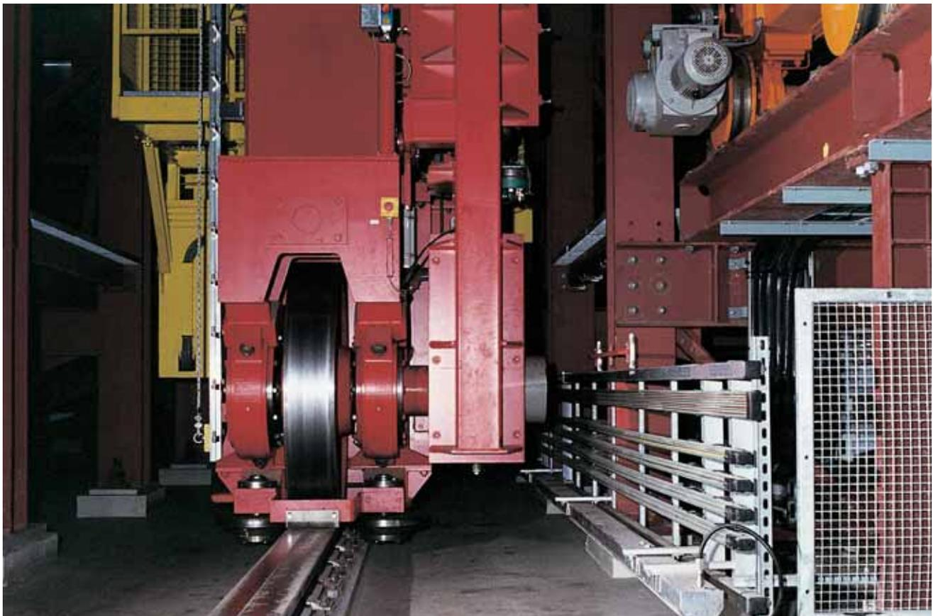
SMG-Data Transmission with VAHLE Conductor System for AS/AR warehouse
